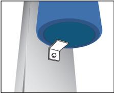
2. If you are mounting a cylinder, make sure the bottom is on a floor, deck or shelf. Alternatively, support it with a piece of angle iron or wood block (see illustration). This makes it easier to tighten the straps with two hands.
