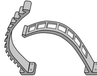
1. The two pieces of the clamp must be mounted with each side facing as illustrated and with the arrows on each base facing each other. Use four #10 bolts or screws and appropriate size washers to fasten each base. Do not over tighten.
